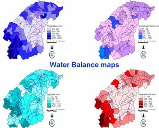
**Fig. 1** Water Balance maps; SWAT output
